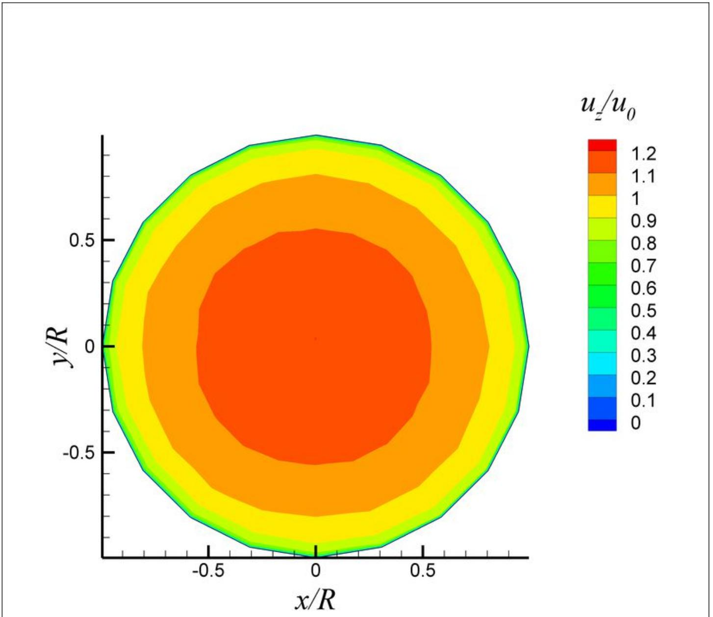
Result of a laser Doppler anemometry measurement on the PTB's heat meter test rig
