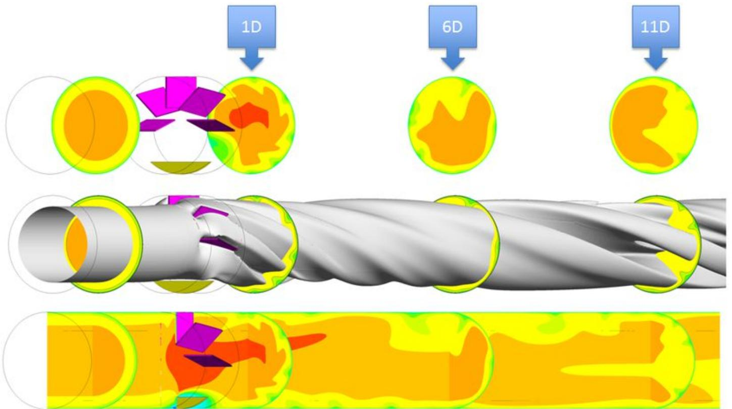
CFD simulation of the flow profile development behind a baffle that simulates an out-of-plane double bend. A fully-formed flow profile flows through the baffle
